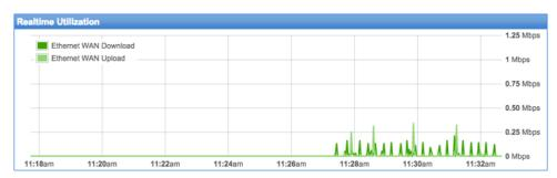
Monitor the past 15 minutes of bandwidth activity on the Usage tab of the Control Panel. Speeds will be indicated on the graph, and each individual Internet Connector will be color coded with Download and Upload separated by shade of color.
