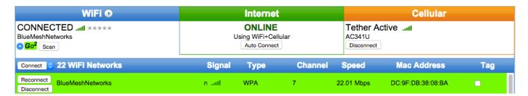
On the Main tab, all active internet sources will display under the Internet Status which indicates that these sources are Load Balancing.
