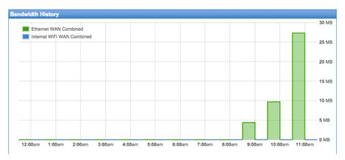
Analyze past consumption of data on the Usage tab of the Control Panel. History is broken out by Internet Connector using color coding. The desired history to display can be changed using various drop-down options below the graph. A table of usage will display by clicking the Show History button on the right. This table can also be downloaded as a CSV export.
