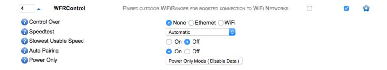
Power Only Mode is used only in troubleshooting situations which require the outdoor unit to be powered up by the indoor router, but not to have data interconnectivity. This mode is helpful when encountering trouble pairing WFRControl, allowing direct access to the outdoor unit's wireless network and Control Panel so that it can be reset to factory defaults before attempting pairing again.
