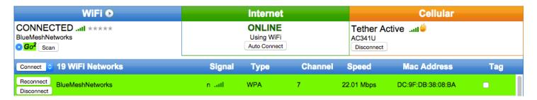
On the Main tab, any backup connections will be highlighted in orange or have an orange flame icon next to them, indicating that they are ready for immediate switchover in case the primary internet source fails.
