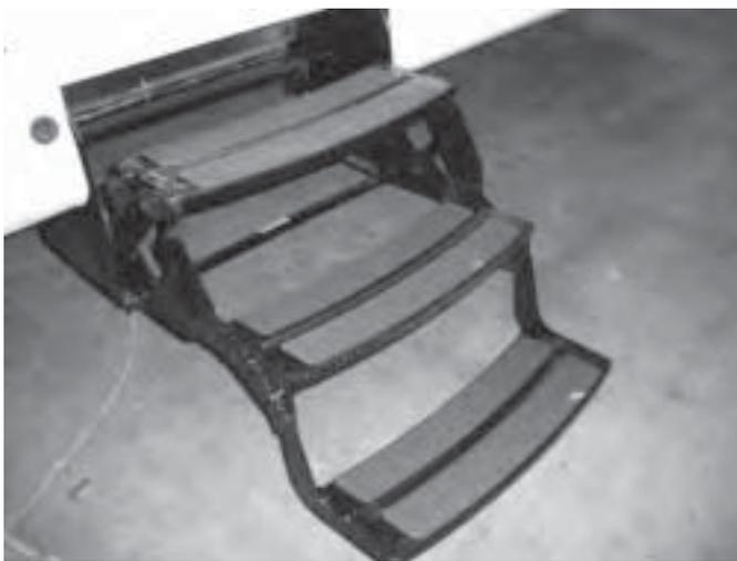
2. Rotate the step elements out and downward.
