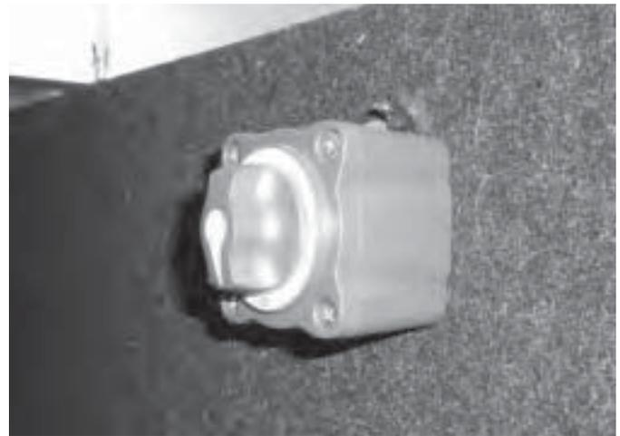
Some accessories or equipment in the trailer may draw small amounts of current even when turned OFF. A battery disconnect (or "load disconnect") system allows you to disconnect the house batteries. Disconnecting
