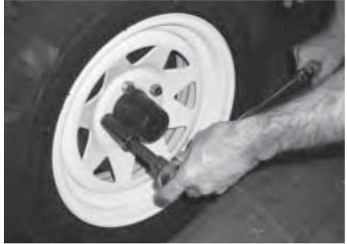
6. Loosen the wheel nuts on the flat tire.
