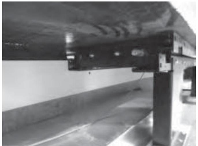
The Happi-Jac electric above floor slide system can be extended or retracted manually using a  $\frac{3}{4}$ " socket and ratchet tool. To retract the room, remove the access panel generally located below the sofa or dinette seat. Place the socket on the shaft connected to the motor and gear mechanism and turn clockwise to extend the room or counter clockwise to retract it. Once the room is retracted it is advisable to secure the room in with travel locks.
