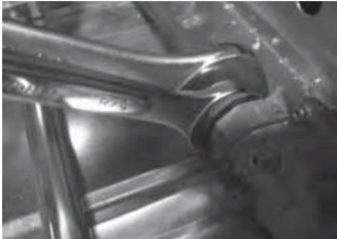
Always tighten flared fittings with two wrenches with opposing torque and do not over tighten. Using only one wrench or over tightening can cause leaks. Have someone stand by to close the main propane tank valve(s) while you are tightening fittings in case a leak occurs. After tightening, check again with the leak detection solution to be sure the leak is stopped. If bubbles still appear, your dealer or a gas service center may need to fix the problem.
