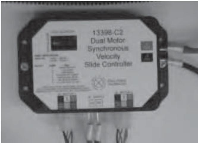
This system utilizes four electric motors and gear systems. The system is operated by an electronic control unit. There is one for each slide room. This control can be tested using the error code or troubleshooting information located on the control itself. There is also a web site that will assist with helping you retract the room
