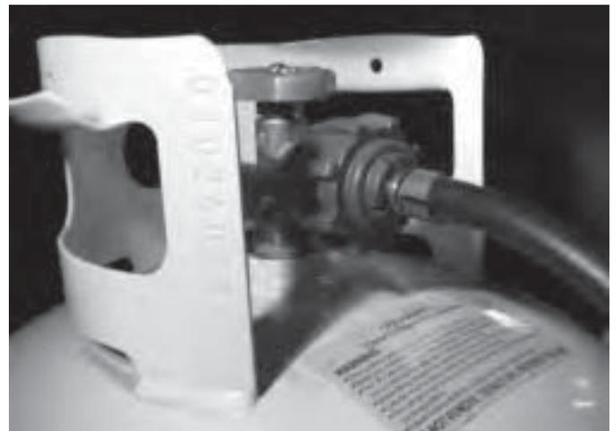
The safety features of this system prevent gas from flowing unless the connection is tight and will limit excessive gas flow. In cases of extreme heat, 240° to 300°F, at the connection, the connection to the cylinder will be shut down.
