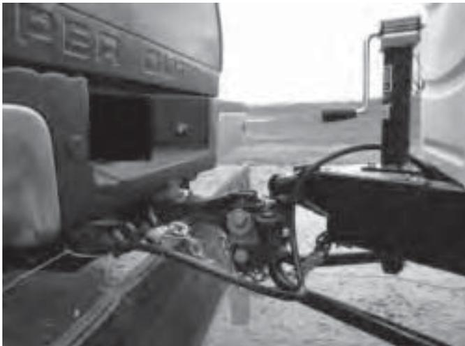
10. Connect the 7-way power cord to the tow vehicle receptacle and the breakaway switch lanyard to a non-removable part of the hitch or the tow vehicle chassis.
