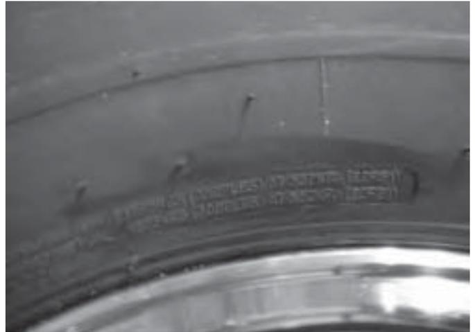
The tire manufacturer's recommended inflation pressure is stamped on the sidewall of the tire. The maximum tire pressure is also listed on the trailer VIN label. Check the tires frequently to be sure they are properly inflated. Always check tire pressure when the tires are cold. Check that the air pressure is equal in all tires. When replacing tires, make sure the replacement tire is the same size and load capacity as the original. See the "Tires and Wheels" chapter for more information.
