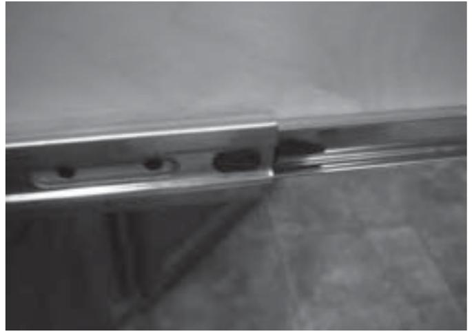
The drawers run in metal guides. To remove a drawer, pull it out until it stops. On each side of the drawer is a latching mechanism. Press the latch while pulling the drawer out slightly to clear the latch tab (ball bearing drawer guides only). Pull the drawer out and lift slightly to clear the guide wheels.
