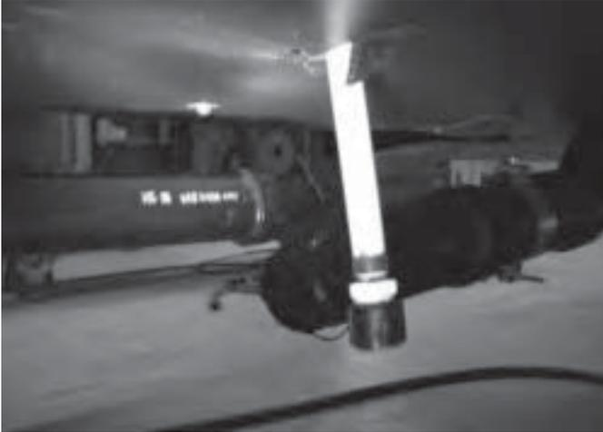
Open the tank drain valve to drain the fresh water tank. If you have a full or nearly full tank, be prepared for the full capacity of the tank to drain. Close the valve when the tank is completely drained.
