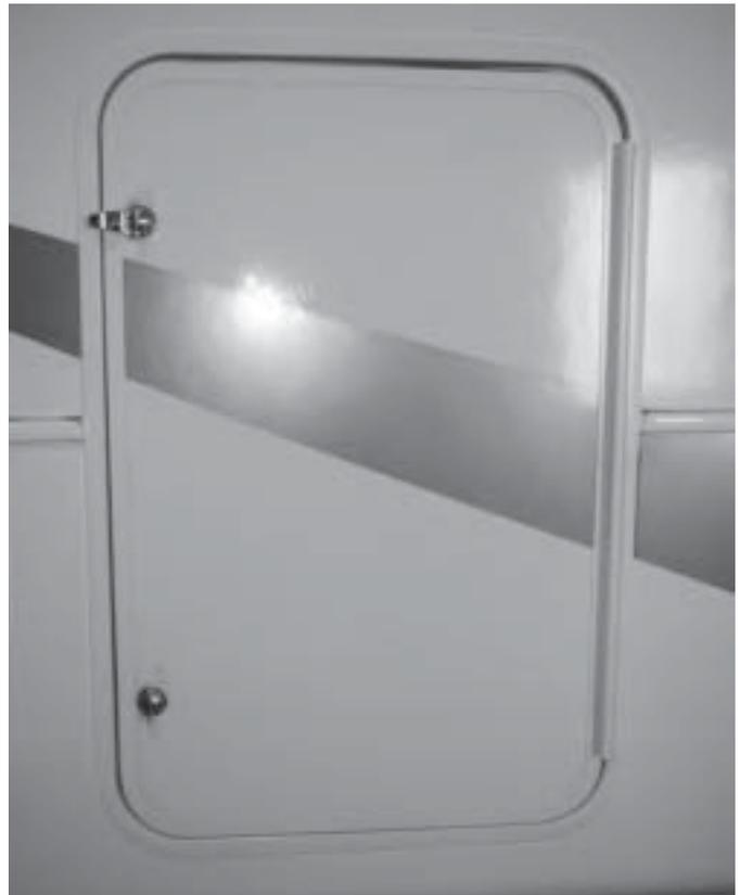
A firm tug on the door at the opposite corner from any binding can almost always eliminate this problem. Another technique is to use a mallet and block of wood to remove any slight interference. During the course
