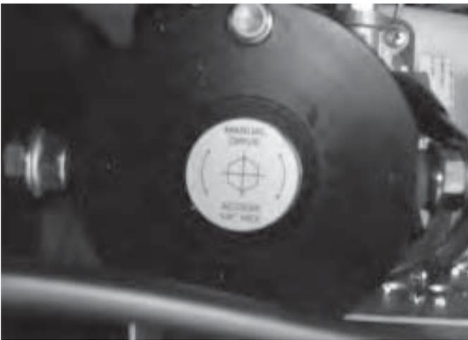
This system uses a hydraulic cylinder and a pump to push the slide room in and out. The system is activated by using a remote control device. As with the other slide mechanisms, it is possible to retract the room manually by installing an electric and/or battery driver into the socket on the pump and manually driving the pump. The pump will be driven clockwise for extend and counter clockwise for retraction.
