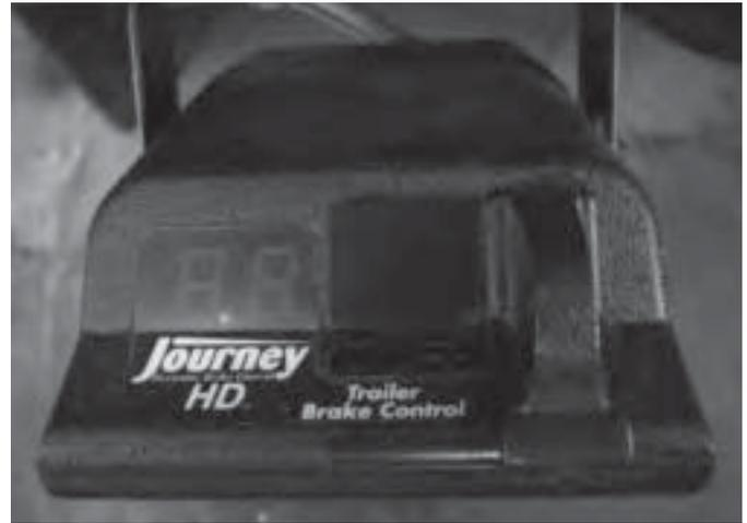
The brake controller (not supplied with your RV) is activated when you apply the tow vehicle brakes. This sends an electrical current to the trailer brakes. You can also apply the trailer brakes independently from the tow vehicle by operating the brake controller by hand. Under normal conditions, you should not operate the trailer brakes by hand, but you have the option when it is needed. See the operating instructions for your brake controller for more information.
