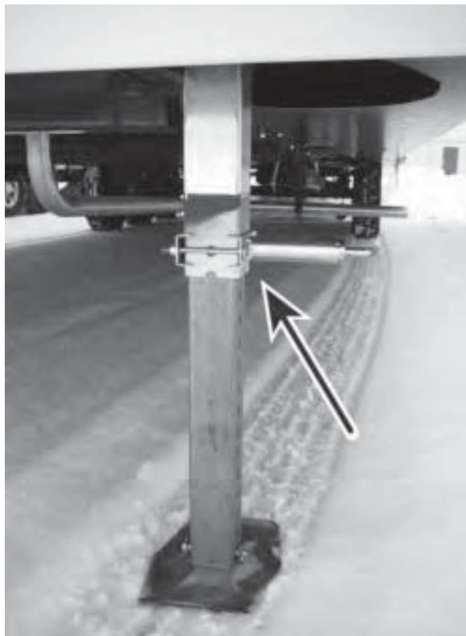
Pull the lock pin on the landing gear leg and allow the drop tube to drop to the ground. Adjust the tube up or down so you can re-engage or re-pin in the nearest adjustment hole.
