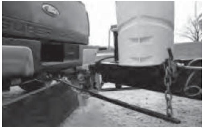
Use a sway control system installed and adjusted according to the sway control manufacturer's instructions. Refer to the hitch installation instructions for detailed preliminary ball mount adjustments.
