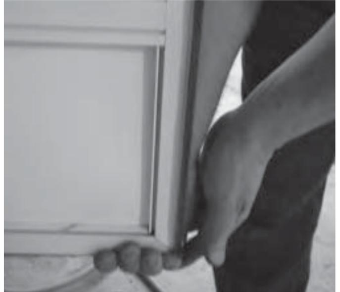
Normal operation and over the road dynamics will cause the screen door hinges to settle slightly, causing the screen frame to drag on the threshold.
