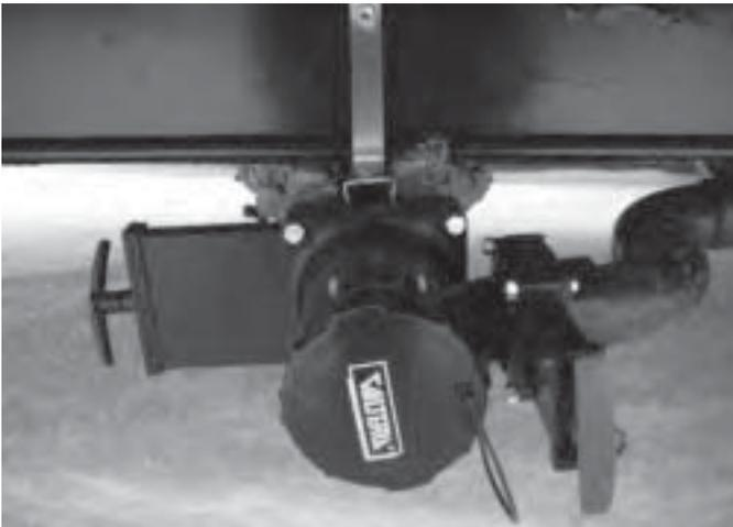
Drain the holding tanks only when they are at least 3/4-full. If necessary, fill the tanks with water to 3/4-full. This provides sufficient liquid to allow complete flushing of waste material into the sewer line.
