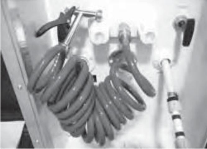
Disconnect the outside shower hose (if equipped) and drain the hose. After all water is drained from the hose, reconnect hose.
