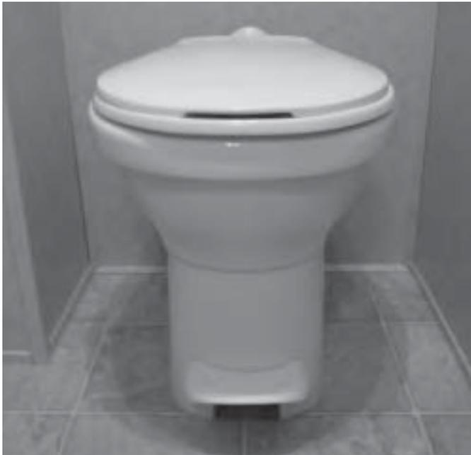
Your trailer is equipped with a marine/RV-type toilet. It operates from water supplied either by the fresh water tank or from an exterior water supply connected at the city water hook-up. (The water pump must be turned on when utilizing the water from the fresh water tank.) The toilet flushes directly into the black water tank. Most models have pedals or hand-operated levers that operate independently. One opens a water valve to fill the bowl, the other operates the valve in the bottom of
