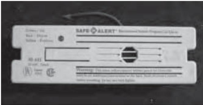
Please refer to the manufacturer instructions supplied with the unit for care and operation of the propane gas leak detector. It is a safety device that is permanently mounted near the floor and is powered by 12V (the RV battery and/or converter). The detector is operational only as long as 12V power is available. If the power is disconnected, the monitor will not operate.
