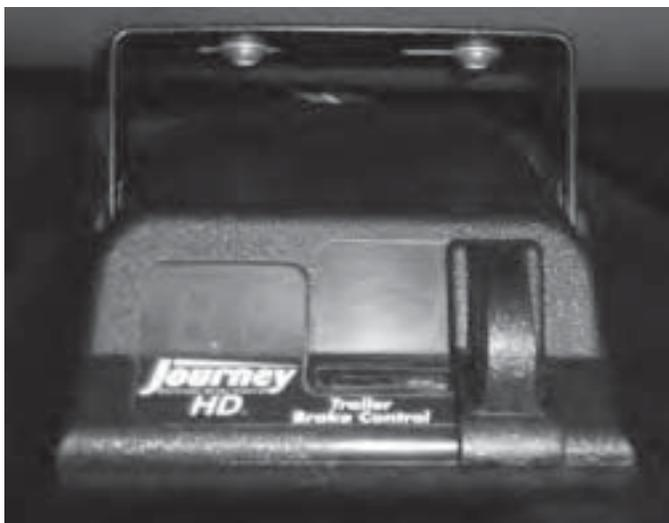
Use a brake controller that automatically applies the brakes in proportion to the tow vehicle brakes and also has a hand control for applying the trailer brakes only. Use outside mirrors installed and adjusted to allow a clear view of the area at both sides of and behind the trailer. Locate them as close as possible to the driver to provide the maximum field of view.
